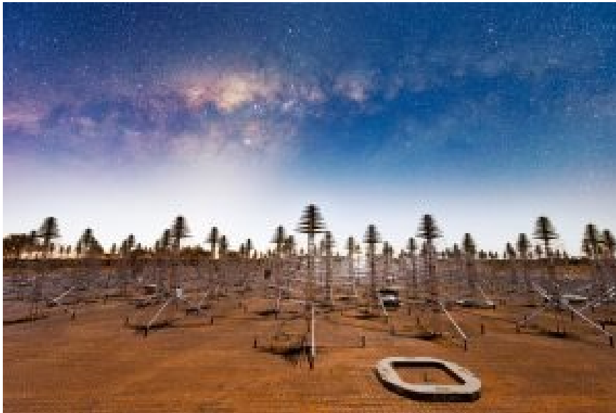
Caption: SKA prototype dipole antennas in a test SKA station (credit: Goh/ICRAR)
