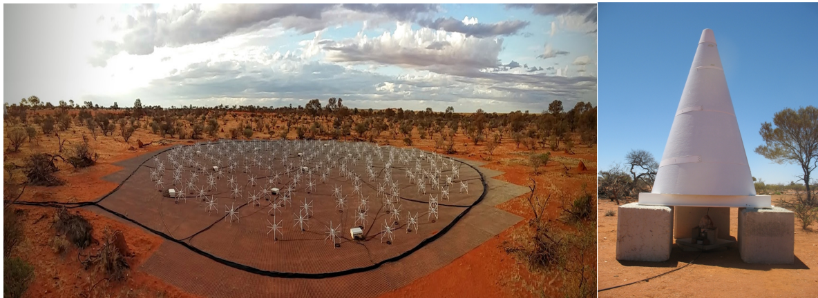
Left : Engineering Development Array (EDA) at the Murchison Radio-astronomy Observatory. Right : BIGHORNS total power radiometer enabling calibration of flux densities in the absolute units.
