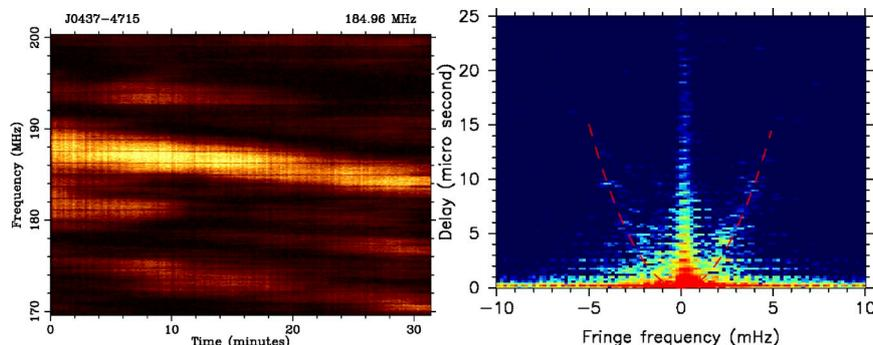
Fig 1: Dynamic scintillation spectrum of the millisecond pulsar J0437-4715 (left) and its secondary spectrum (right), from MWA observations (Bhat et al. 2018). Faint *parabolic arc-like* features arise from the deflected parts of pulsar’s scattered radiation. The indicated delays (~microseconds) will be directly measurable using the new capabilities and the advanced techniques that will be realised through this project.
