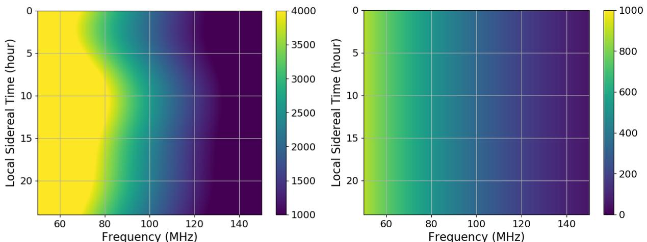
Left: A simulated data set showing the radio continuum background measured by a single element radio telescope over 24 hours. Right: The isotropic component isolated from the radio background data using the initial algorithm which will be developed further as a part of this project.
